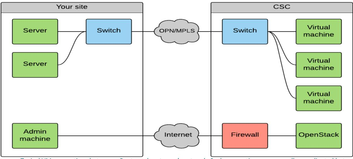
Typical VM connections between ePouta and customer's network. Such connections are normally coordinated between CSC's cloud team, Funet and customers IT department for initial setup.
