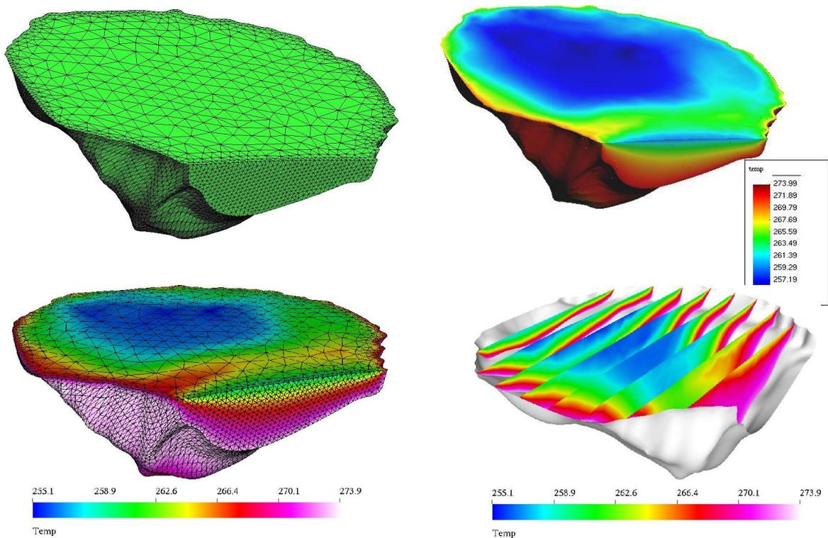
Figure 2: Modeled temperature distributions in a crater glacier. Element mesh in GiD (top left), results in GiD postprocessor (top right), and results in ElmerPost (bottom left and right). The mesh was generated in GiD, the simulations were performed with Elmer and the results have been visualized both with GiD and with ElmerPost. The temperatures above are given in Kelvin.
